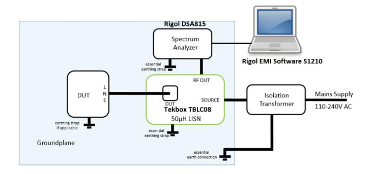
The setup is not standard conformant, given the available space may be limited. In case that there is sufficient space, the relevant CISPR or EN standards contain descriptions and pictures of standard conformant set-ups. It is essential to use an isolation transformer for any  $50\mu$ H LISN. The internal capacitors draw much blind current and would cause the ground protection switch to trip without isolation transformer.
