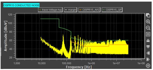
The conducted emissions of the LED flood light measured with Average detector significantly exceed the limit line (orange).
