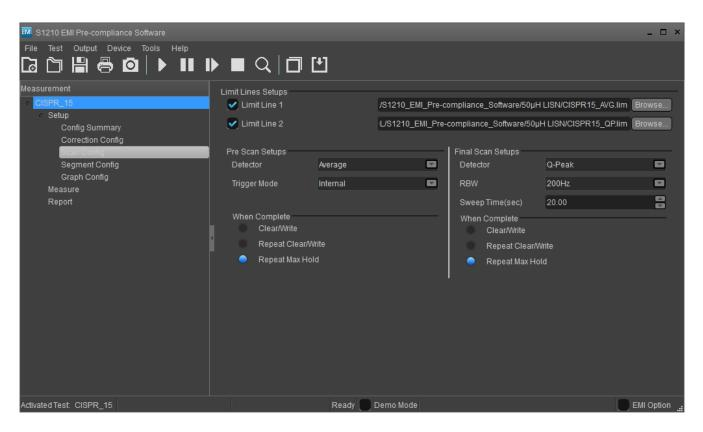
In *Pre Scan Setups* set *Detector* to *Average*, *Trigger mode* to *Internal* and *Repeat Max Hold*. In *Final Scan Setups* set the *RBW* to 200Hz and the *Sweep time* to 20 seconds (according to chapter 3).
