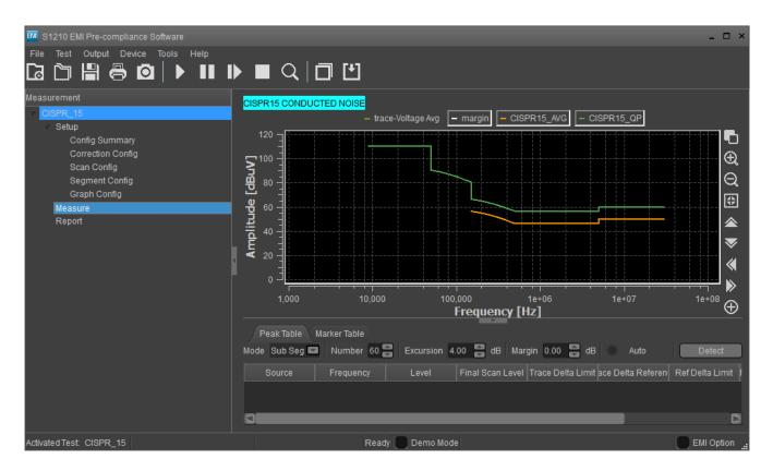
Note that the S1210 SW does not display beveled limit lines according to the standards.
