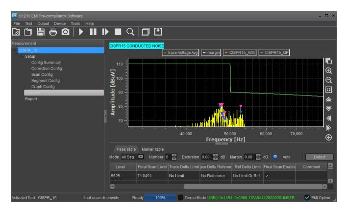
The measurement result was then displayed with blue triangles. The final scan of the conducted emissions with Quasi Peak detector showed that the Philips LED tube was within the CISPR 15 limits again.
