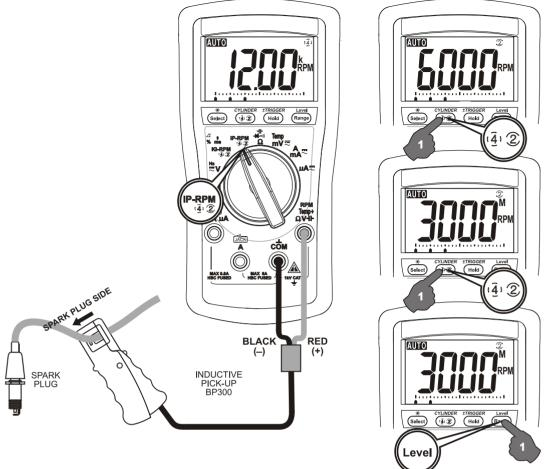
Press (4.2) button momentarily to select through **RPM**<sup>4</sup>  $\frac{3}{2}$  for 4-stroke, **RPM**<sup>2</sup> for 2-stroke and DIS, and **RPM**<sup>2</sup> **M** for special 2-stroke waste ignition engine
