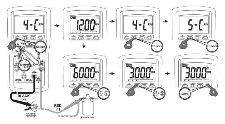
Press (4.2) button momentarily to select through **RPM**<sup>1</sup>(4.2) for 4-stroke, **RPM**<sup>2</sup> for 2-stroke and DIS, and **RPM**<sup>2</sup> **M** for special 2-stroke waste ignition engine
