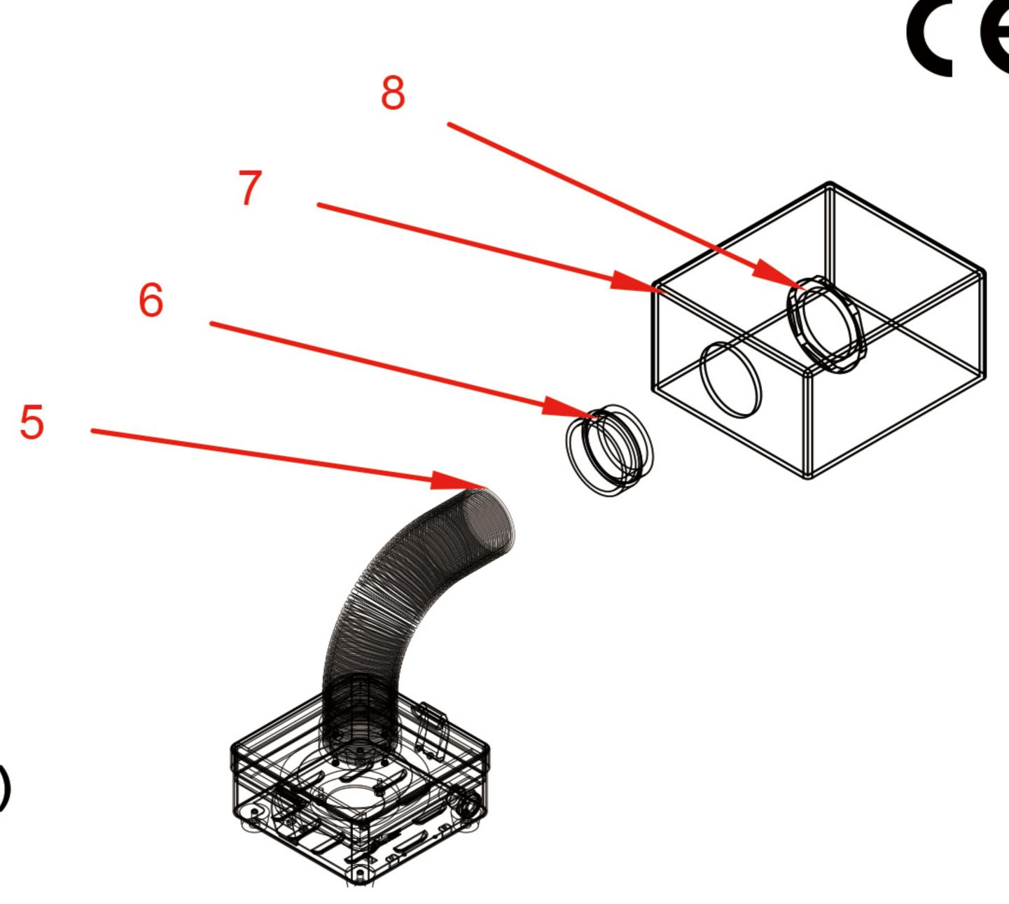
3.Insert the "5" knob into "6", insert the other end of "6" into the round hole of "7", and use "8" to tighten "6" from inside "7"
