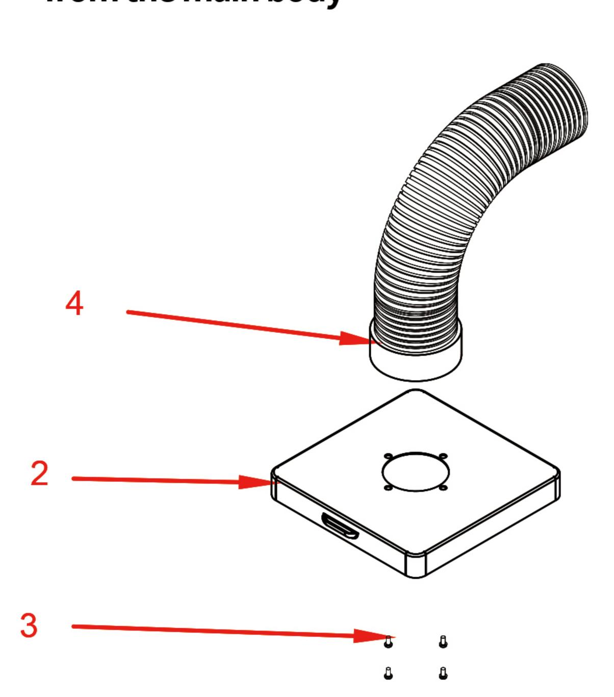
2.Place "4" on the upper surface of "2" and align the screw holes, use four screws ("3") to tighten "1" from the bottom of "2"
