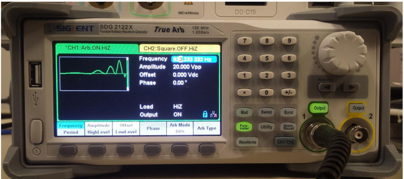
Connect the AWG channel to an oscilloscope and verify that it meets the application requirements. You can adjust the waveform amplitude, frequency, Arb Mode, and other features from the front panel of the AWG if it requires fine-tuning.
