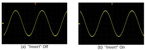
Figure 2-1 Waveform Invert
