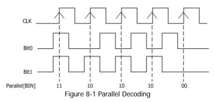
Press MATH → Decode1 → Decoder to select "Parallel" and open the parallel decoding function menu.
