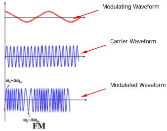
Figure 13-11 Frequency Modulation
