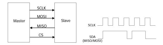
Figure 8-1 SPI Serial Bus
