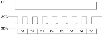
Figure 5-15 Sequential Chart of SPI Bus
