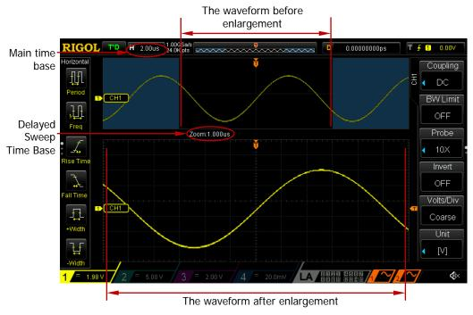
Figure 3-1 Delayed Sweep Mode
