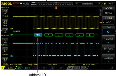
Figure 8-6 I2C Address Information during Decoding
