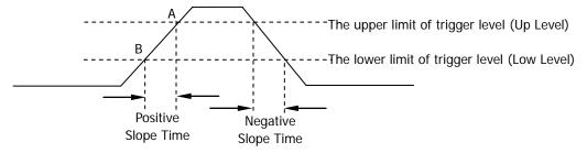
Figure 5-4 Positive Slope Time/Negative Slope Time
