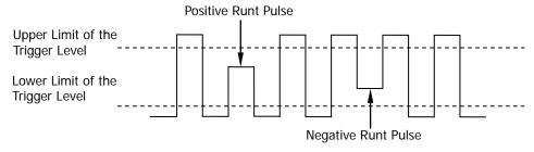
Figure 5-9 Runt Trigger
