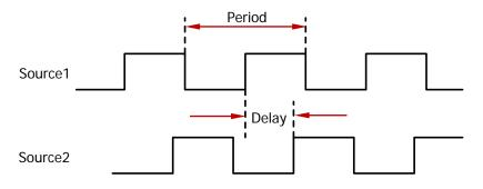
Figure 6-4 Delay and Phase
