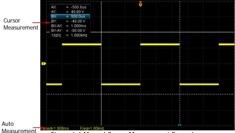
Figure 6-6 Manual Cursor Measurement Example
