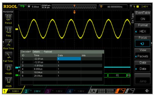
Figure 8-2 Parallel Decoding Event Table
