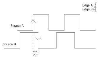
Figure 5-10 Delay Trigger
