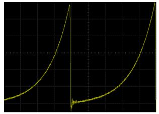
Figure 13-4 Built-in Waveform-ExpRise
