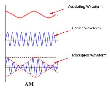
Figure 13-10 Amplitude Modulation
