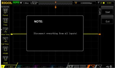
Figure 15-2 Self-calibration Interface
