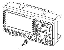
Figure 1-5 To Connect the Passive Probe
