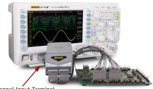
Digital Channel Input Terminal Figure 1-6 To Connect the Logic Probe
