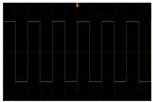
Figure 4-2 The Waveform after 256 Averages
