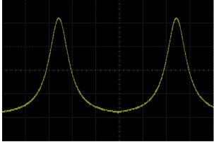
Figure 13-8 Built-in Waveform-Lorentz
