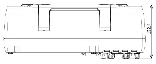
Figure 1-2 Top View Unit: mm
