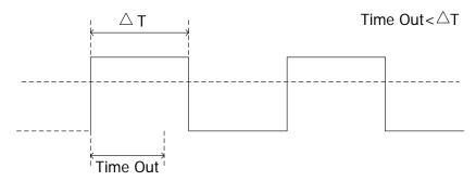
Figure 5-8 TimeOut Trigger
