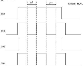
Figure 5-7 Duration Trigger
