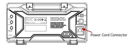
Figure 1-4 To Connect to Power Supply
