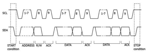
Figure 5-14 Schematic Diagram of I2C Protocol
