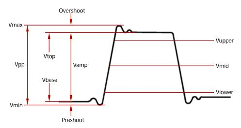
Figure 6-5 Voltage Parameters
