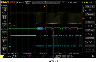
Figure 8-7 I2C Error Expressions during Decoding
