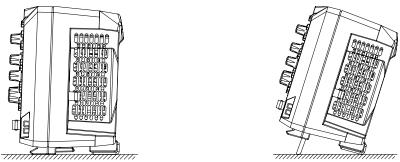
Figure 1-3 To Adjust the Supporting Legs
