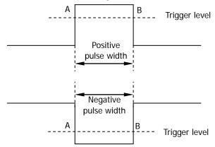
Figure 5-3 Positive Pulse Width/Negative Pulse Width
