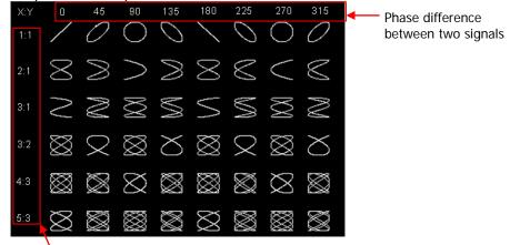
Frequency ratio between two signals
