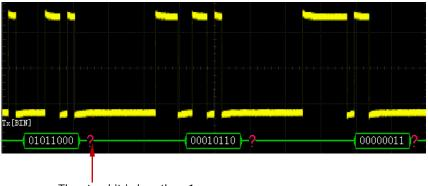
The stop bit is less than 1
