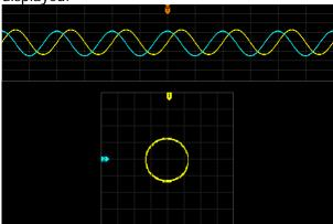
5. Observe the measurement result shown in the figure above. According to the measurement schematic diagram of the phase deviation (as shown in Figure 3-2), A/B (C/D) = 1. Thus, the phase deviation angle  $\theta$ =±arcsin1=90°.
