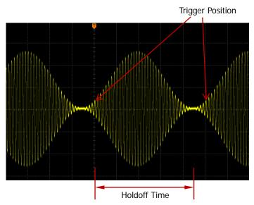
Figure 5-2 Schematic Diagram of Trigger Holdoff
