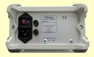
The circuit used, conforms to the specifications of EN 55016-1-2, VDE 0876 and ANSI C63.4 for V-networks with a simulated impedance of (50µH / 250µH + 5  $\Omega$ ) || 50  $\Omega$  in the frequency range 9 kHz to 30 MHz.
