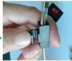
3. Remove the damaged fuse with a screwdriver
