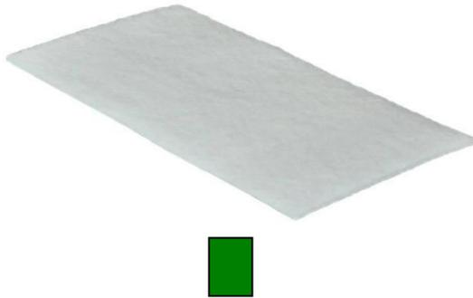
Use method: Place the Pre-filter on top of the Middle Filter. The front side (rough side) is facing upwards (air inlet direction). When the accumulated dust on the Pre-filter is over 70% and cannot be cleaned any more, please replace the Pre-filter with a new one.
