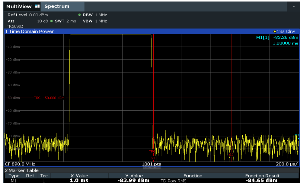
Figure 6-19: Measurement of the signal-to-noise ratio of a GSM burst signal in zero span
