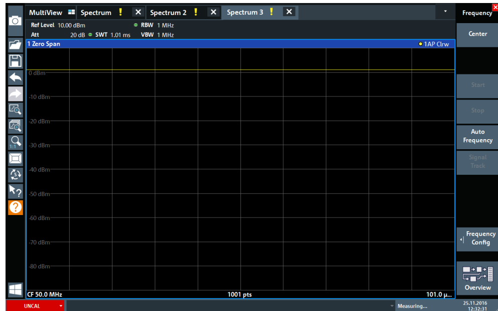
Figure 4-10: Time domain display of the calibration signal
