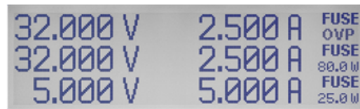
Figure 4-6: Overvoltage protection (example R&S HMP2030)
