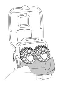
Remove the solder collection tray for disposal of solder waste.
