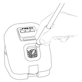
The CLMU-A is automatically switched off if the splashguard is opened during operation.
