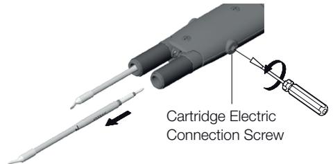
**Important:** It is essential to insert the cartridge till the end for a good connection. Take the mark as reference and check that both tips of the tweezers coincide.
