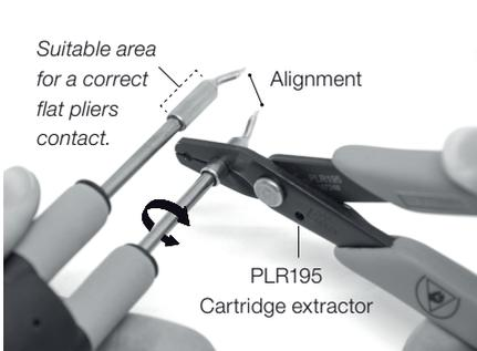
Use a flat pliers in the indicated area for a correct tip alignment.
