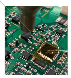
IPC\* does not recommend exceeding ramp-up rates over  $3-4^{\circ}\text{C}$  / sec. (5-7°F / sec) so as to reduce the risk of thermal stress on the PCB.
