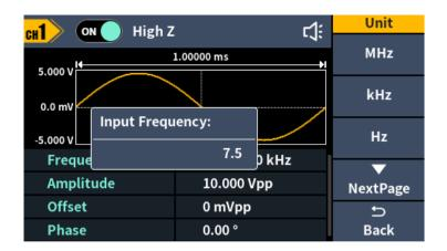
Figure 4-4: Use numeric keypad to set the frequency
