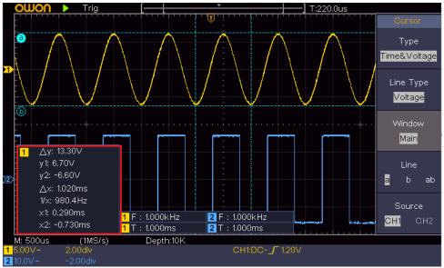
Figure 4-15 Time&Voltage Cursor Measurement
