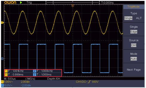
Figure 4-12 Automatic measurement
