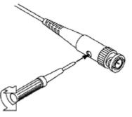
Figure 3-7 Adjust Probe
