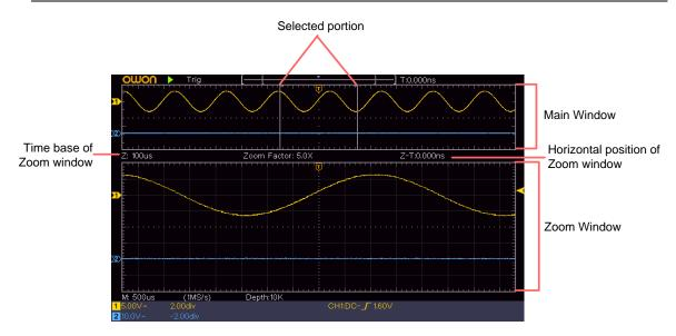
In normal mode, the **Horizontal Position** and **Horizontal Scale** knobs are used to adjust the horizontal position and time base of the Main window.
