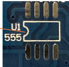
1x Single precision timer (IC) On the PCB: U1 Pay attention to the orientation:
