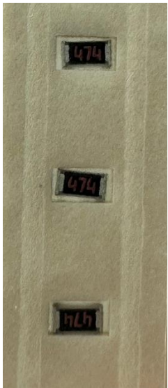
14x (or more) 0603 size resistor On the PCB: R34-R47
