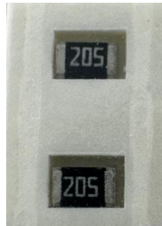
1x (or more) 0805 size 2MΩ resistor On the PCB: R49
