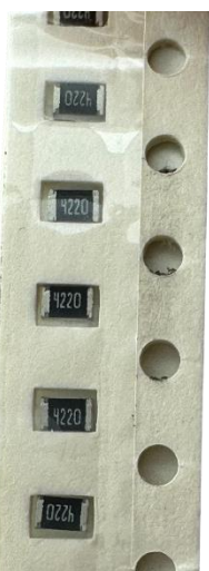
15 (or more) 0805 size resistor On the PCB: R50-R60/R65-R68
