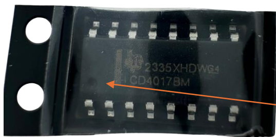
1x Decade counter (IC) On the PCB: U2 Pay attention to the orientation:
