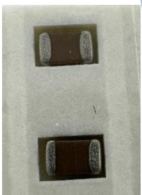
2x 0805 size 0.1uF capacitor On the PCB: C27-C28
