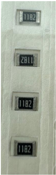
12x (or more) 0805 size resistor On the PCB: R13-R24
