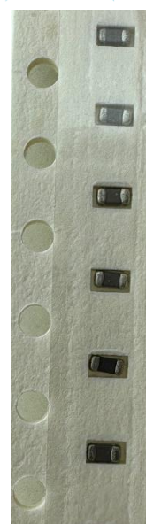
14x (or more) 0603 size capacitor On the PCB: C13-C26
