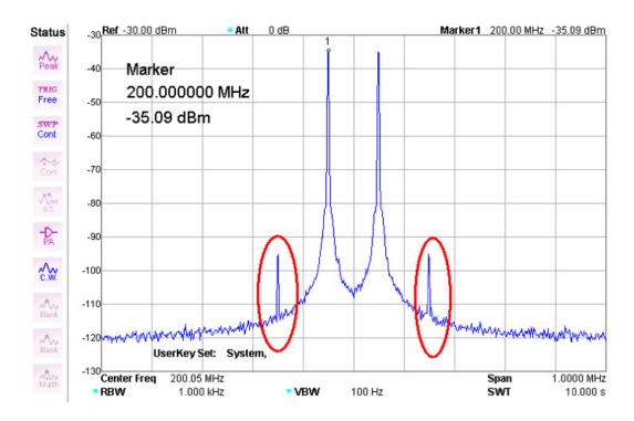
The following spectrum shows the spectrum of the same set up, however using the TBHDR1 pre-amplifier instead of the internal amplifier of the analyzer. Due to the high IP3 of the TBHDR1, the amplitude of
