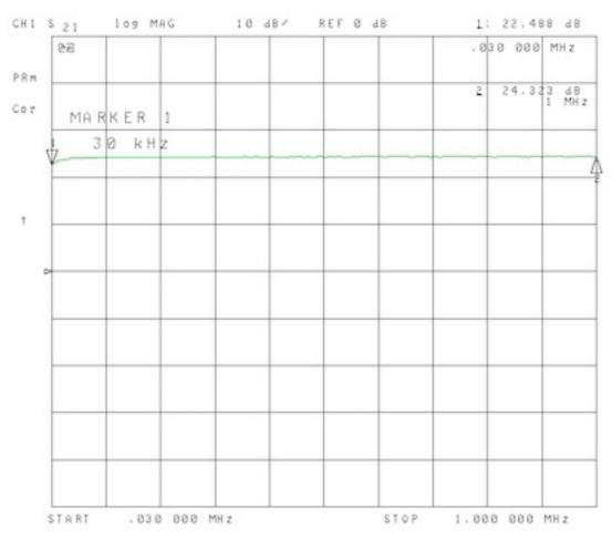
Picture 3 - TBHDR1, gain, 30 kHz - 1 MHz
