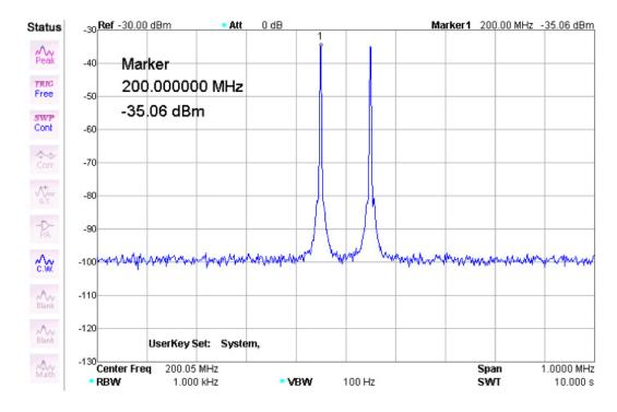
If there is no requirement to look at signals with amplitudes close to the noise floor, everything is fine. However, if the spectrum has to be checked for signals with amplitudes close to the noise floor of approximately -100 dBm, the internal pre-amplifier of the spectrum analyzer needs to be turned on.
