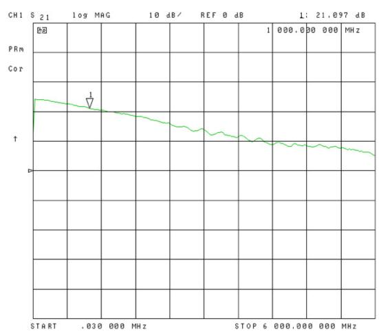
Picture 5 - TBHDR1, gain, 30 kHz - 6 GHz
