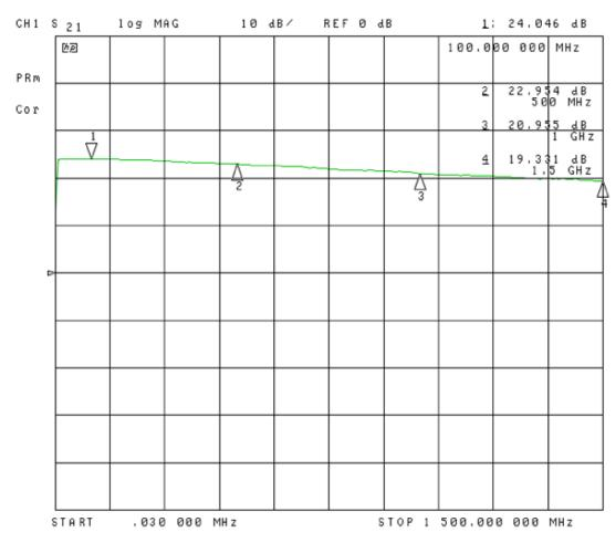
Picture 4 - TBHDR1, gain, 30 kHz - 1.5 GHz
