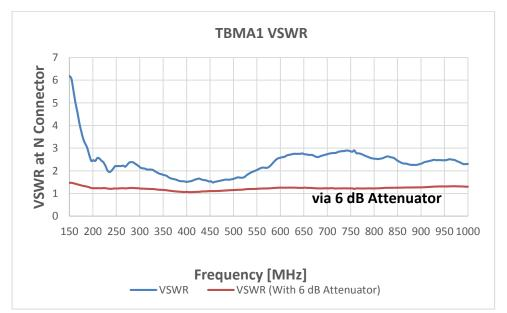
Picture 16 – 150 MHz...1 GHz , Measured VSWR at N Type connector without/ with 6 dB Attenuator
