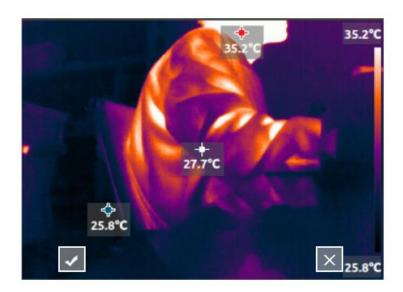
• As shown in the figure below, you can save the thermal image and visible light image by pressing the "trigger button" or "OK & Homepage", and press the "Return & Power" to cancel saving.
