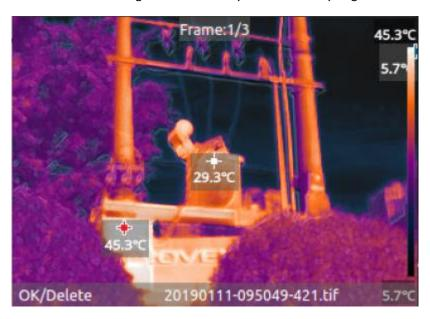
$\circ$  2<sup>nd</sup> frame: the raw image frame of thermal image
