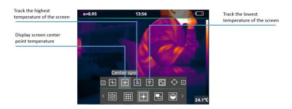
Press the trigger button will freeze the image as the figure below,
