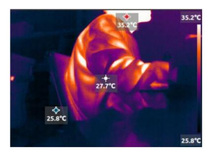
• If the temperature value is not displayed on the screen, press "OK & Homepage", then select the "Measurement" icon , and then select "Center Spot", "Hot Spot" and "Cold Spot" in the figure below to display the temperature,
