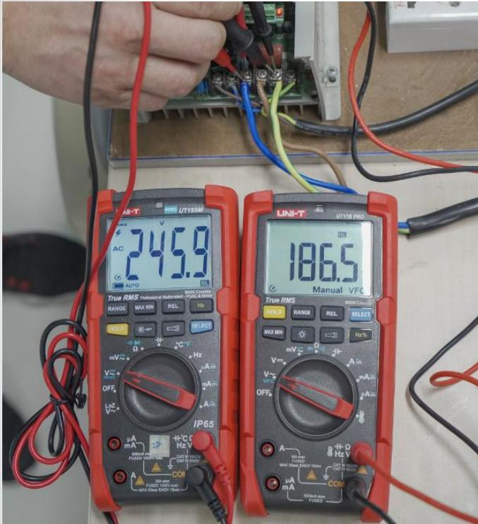
Traditional Non-VFC meter when testing variable frequency (meter on the left in picture) voltage/frequency:
