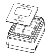
Figure 8. Battery Replacement
