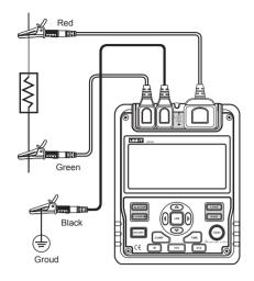
Figure 5. Insulation Resistance Measurement
