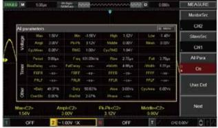
Automatic Measurement of Waveform Parameters
