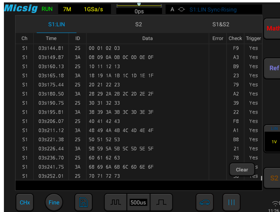
Figure 13-13 LIN Text Interface
