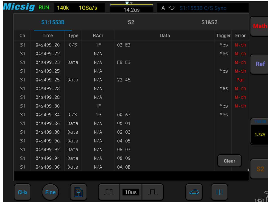
Figure 13-33 1553B Text Interface
