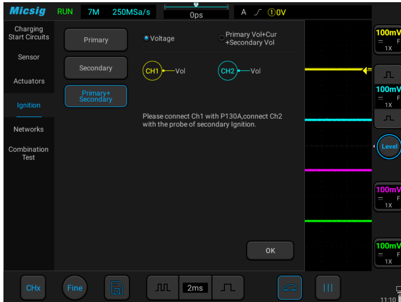
Figure 3-43: Primary + Scndary ignition test
