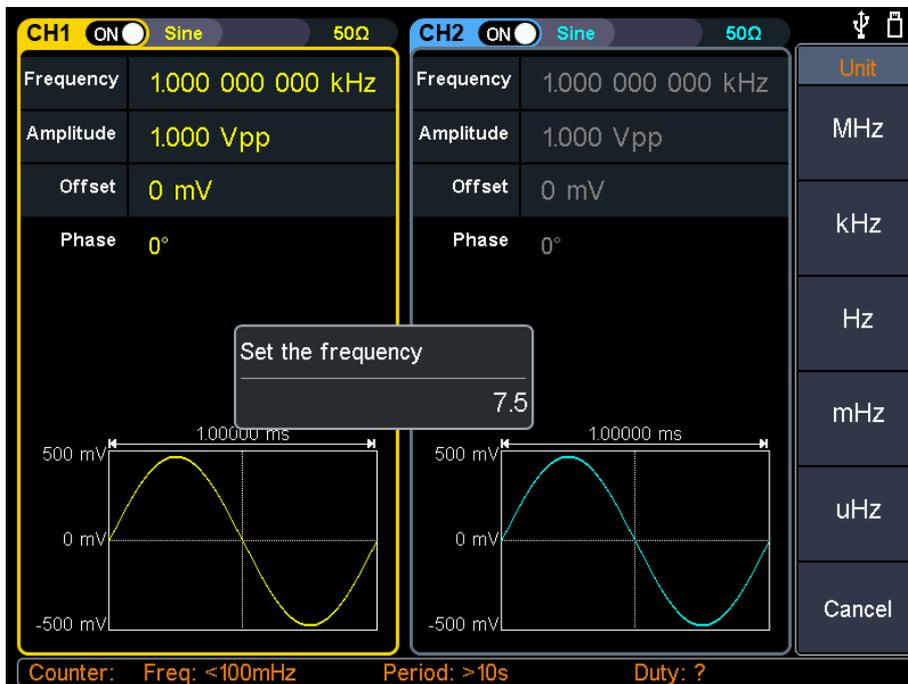
Figure 4-4: Use numeric keypad to set the frequency
