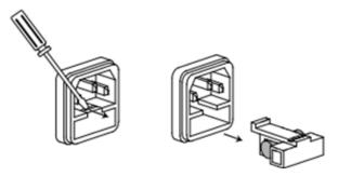
3. Replace the fuse with a new one, install it into the fuse box, and push the fuse box back on to the rear panel.
