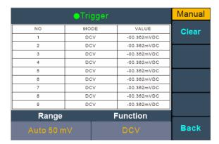
**3.** Clear the manual record: Press the Clear soft key to clear all data in the data table. (Note: because manual and automatic records share the same data table, automatic readings are also erased.).
