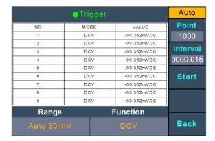
2. Record data: Press the Start softkey to start auto record. The // icon will show up on the top of the display. Press the Stop softkey to stop recording, the data table shows the readings taken. press keys to turn the page.
