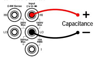
**Tip:** Please short contact the two feet of an electrolytic capacitor by using a test lead before measuring the electrolytic capacitor.
