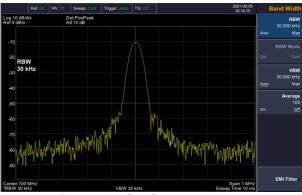
Figure 3-9 Set frequency span
