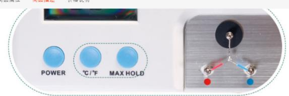
Press the  ${}^{\circ}\text{C}/{}^{\circ}\text{F}$  button and Max Hold button together and hold them for about 5 seconds then release, the meter enters into password inputting mode.(The POWER button is to confirm the data you put in and to bring you to the next data setting. The  ${}^{\circ}\text{C}/{}^{\circ}\text{F}$  and Max Hold buttons are to adjust the value)
