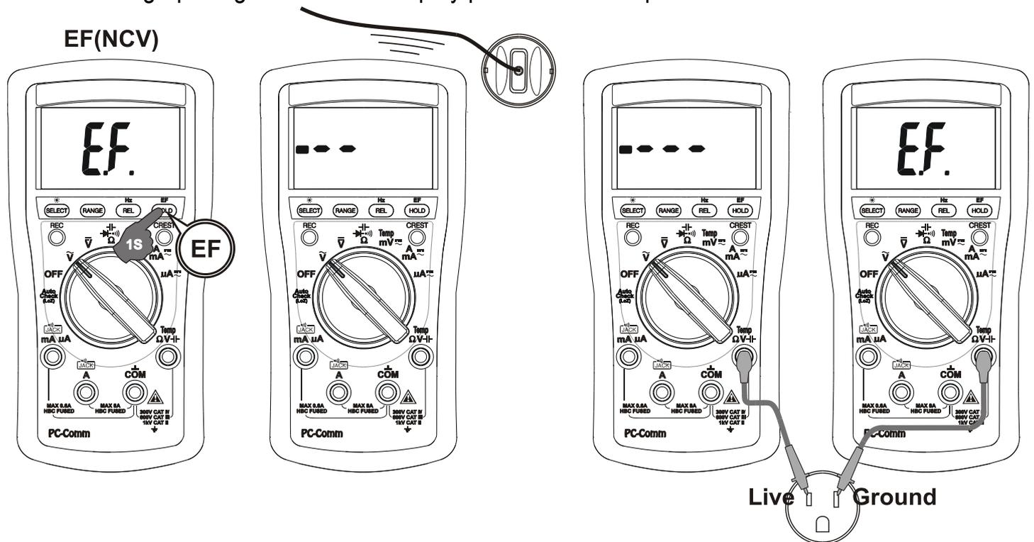
● **Non-Contact EF-Detection:** An antenna is located along the top-right end of the meter, which detects electric field surrounds current-carrying conductors. It is ideal for tracing live wiring connections, locating wiring breakage and to distinguish between live or earth connections.
