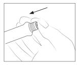
Push the sealing plug inside the handle until the sealing plug and handle edges are aligned.
