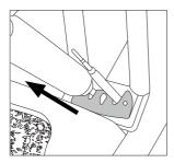
Place the handpiece in the extractor and pull it to remove the cartridge.
