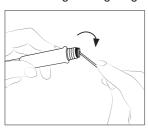
Enter a small shaft or screwdriver, not deeper than 8mm, and lift and pull the sealing plug. Never use a cartridge to do this operation.
