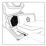
Remove the wiper by pulling it out.
