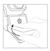
Lift the wiper at its front edge.
