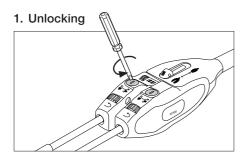
Unlock the fixing screws.
