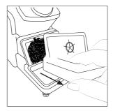
Remove the wiper by pulling it out.
