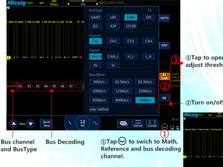
③Tap to open slip bar, slip up and down to adjust threshold value.
