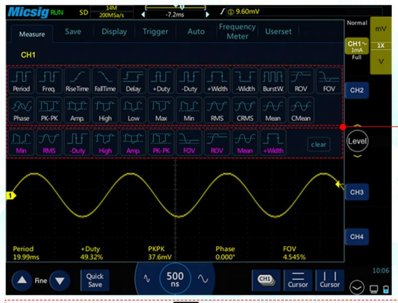
Enabled measurement parameters are displayed here.
