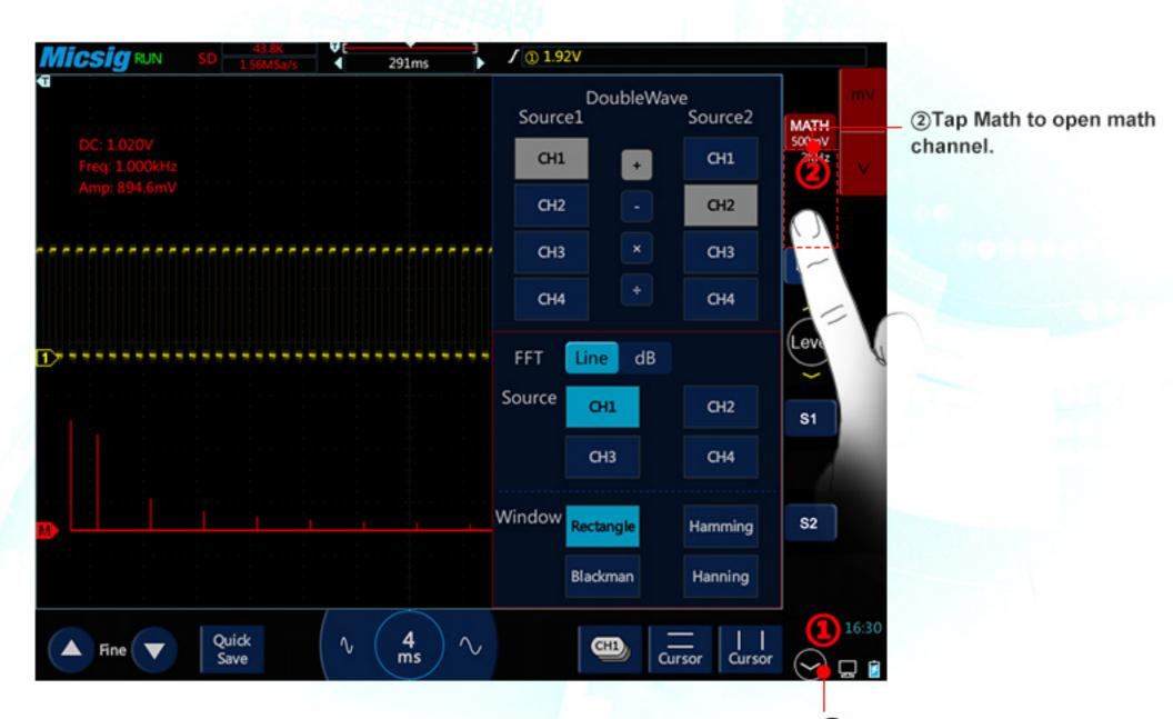
①Tap to switch to Math, Reference and bus decoding channel.
