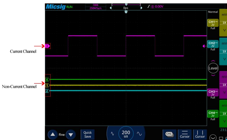
Figure 4-2 Current Channel and Non-Current Channel
