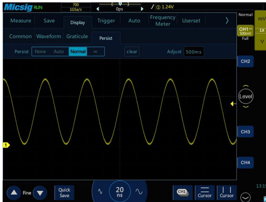
Figure 9-4 20MHz Sine Wave Variable Persistence 500ms
