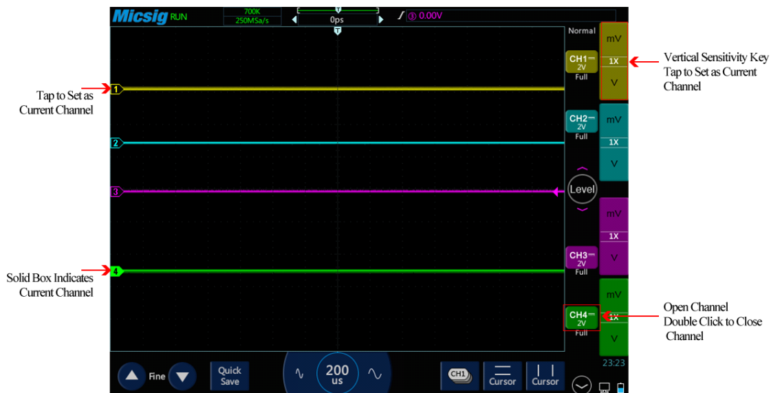
Figure 4-4 Channel Open, Close and Switching
