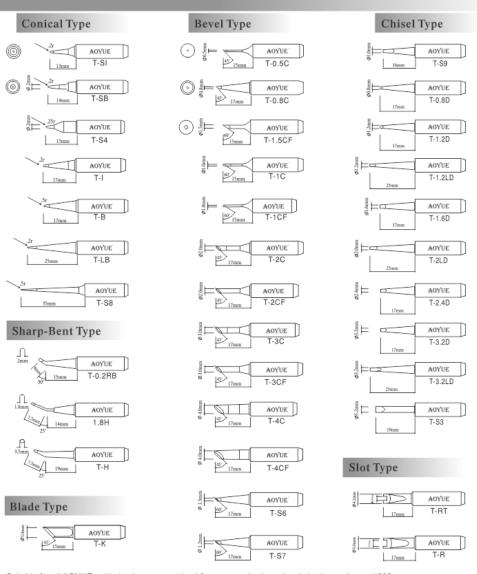
Suitable for all AOYUE soldering irons except lead free composite tip series, induction series and 938
