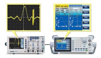
Direct Waveform Reconstruction (DWR) Capability
