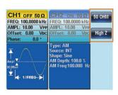
50  $\Omega$  /High Z Impedance Switch Function
