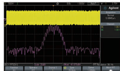
KEYSIGHT DSOX2000A - FFT Display
