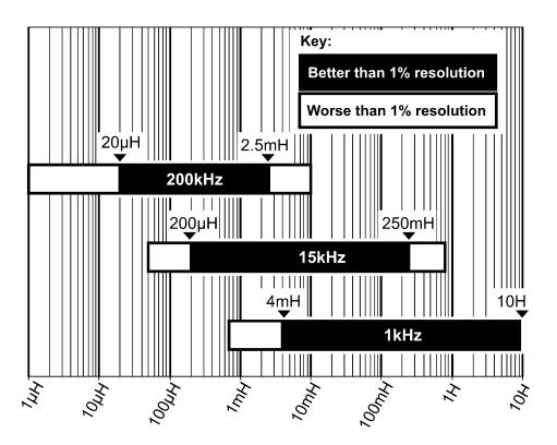
Measuring inductance outside of the black bands will result in degraded measurement resolution (possibly worse than 1% of the measured value).
