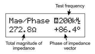
This display is useful for gauging how close your component is to a theoretical "ideal" inductor, capacitor or resistor.
