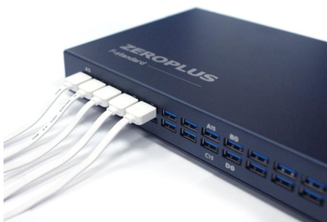
Figure 2-4 Test cables connected to the LAP-F1
