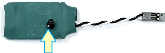
Figure 2-7 eMMC probe tuning screw
