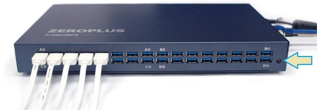
Figure 2-5 Signal cable connection and power lamp location
